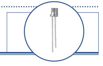
The OPV330 is a Vertical Cavity Surface Emitting Laser (VCSEL) packaged in a flat lens lateral package. VCSELs offer many advantages in sensing applications when compared to infrared LEDs. These devices require substantially lower drive currents to obtain the same amount of output power as LEDs. This feature allows VCSELs to be used in low power consumption applications such as battery operated equipment.
